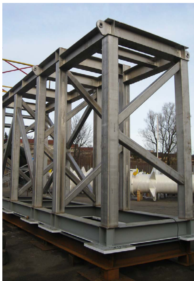
assembled skid 9.3x2.4x8.6m (LxWxH)
