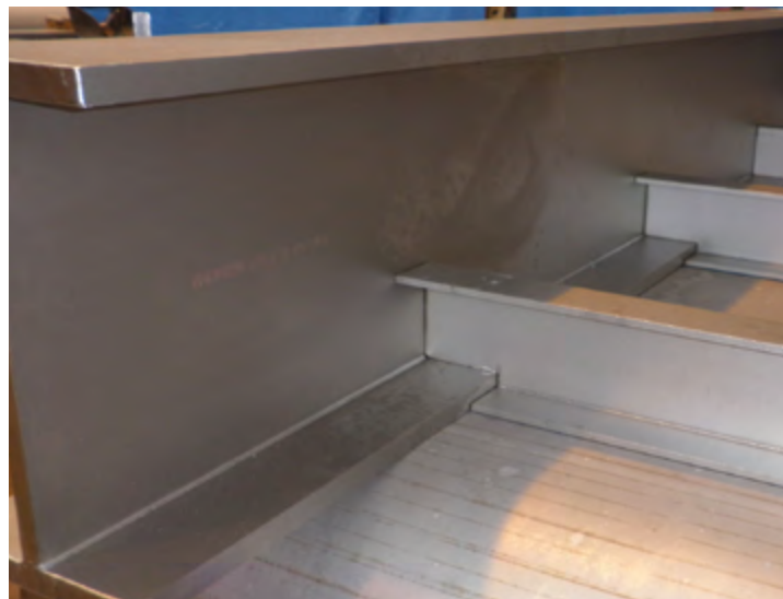
detail with beams composing the structure of a tank module
