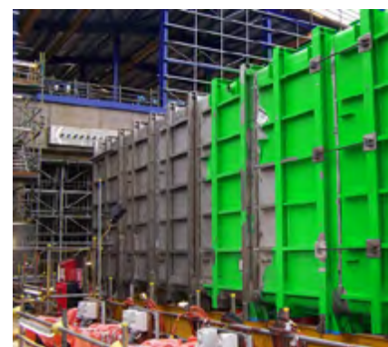
detail with beams composing the structure of a tank module
