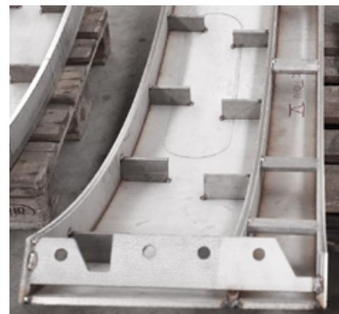
*all base material was laser-cut to shape prior to assembly and fusing*
